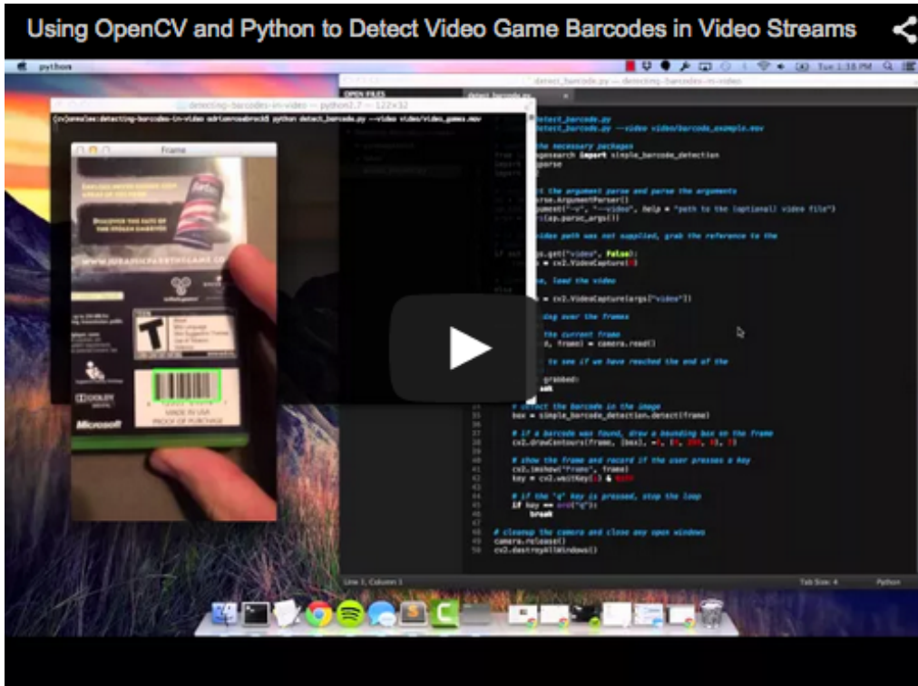
As an example, check out the screenshot below (captured using a video stream from my webcam) of me holding up the back cover of Modern Warfare 3 and the barcode being detected successfully.
